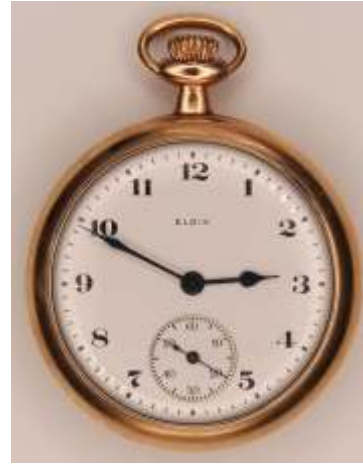
1300 Elgin National Watch Co. vintage pocket watch. Grade 291, model 7, 7 jewels. White enamel face with Arabic numerals and sunk second sweep. Partial plate in nickel. Fahys Montauk Watch Case Co. guaranteed 20 year gold plated. Size 16, serial no. 23404079, circa 1921. Excellent condition, working at the time of cataloguing. Estimate $200 - 300
