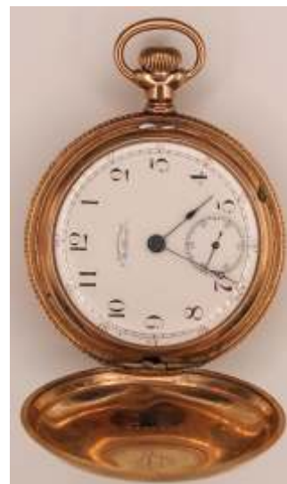
1343 Waltham Watch Co. vintage pocket watch. Grade P.S. Bartlett, model 1883, 17 jewels, side winding. White enamel face with Arabic numerals and double sunk second sweep. Full plate in nickel. Keystone Watch Case Co. gold plated. Size 18, serial no. 7580935, circa 1896. Very good condition, working at the time of cataloguing. Estimate $300 - 400
