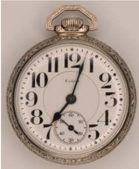
1285 Elgin National Watch Co. vintage pocket watch. Railroad grade 453 Veritas, model 15, 23 jewels. White enamel face with Arabic numerals and double sunk second sweep. Partial plate in nickel. Supreme Illinois Watch Case Co. is nickel plated. Size 16, serial no. 22554547, circa 1920. Excellent condition, working at the time of cataloguing. Estimate $600 - 800
