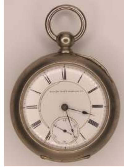
1292 Elgin National Watch Co. vintage pocket watch. Grade 69 B.W. Raymond, model 1, 15 jewels key wind pocket watch. White enamel face (hairlines) with Roman numerals and double sunk second sweep. Partial plate in nickel. Watch case nickel plated. Size 18, serial no. 263647, circa 1873. Very good condition, working at the time of cataloguing includes chain and key. Estimate $300 - 400
