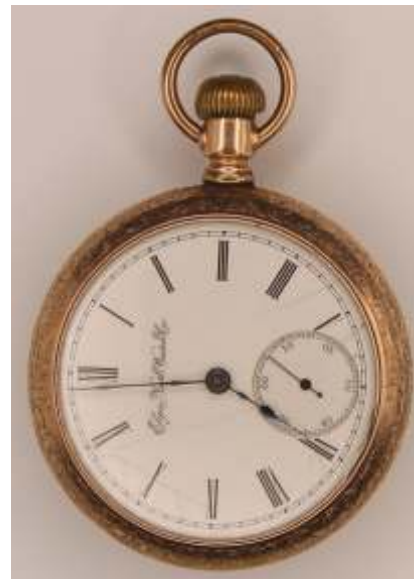
160 Elgin National Watch Co. vintage pocket watch. Grade 33 H.H. Taylor, model 2, 15 jewels. White enamel face (hairline cracks) with Roman numerals and sunk second sweep. Full plate in nickel. Case is gold plated. Size 18, serial no. 4403474, circa 1891. Good condition, working at time of cataloguing. Estimate $100 - 150
