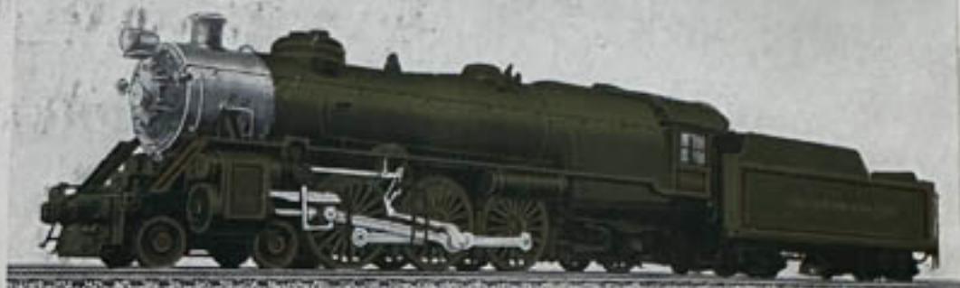
Locomotive No. 5320, "President Cleveland," of the Baltimore and Ohio, which heads the railroad's Air-Conditioned train exhibited at A Century of Progress, Chicago, 1934 Completed in B. & O. Shops, Baltimore, October, 1929. Tractive power, 50,000 pounds. Drivers, 80-inch. Water tube firebox, 503 square feet of heating surface. Total weight of engine and tender, 569,500 pounds. Large drivers, low running board and concealment of piping and light machinery give the President Cleveland a striking appearance. Up until April 30, this locomotive had run more than 420,000 miles
